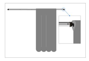
③ String drape onto the Drape Support (CROSSBAR)before hanging\*I like to do 4-5 panels per 10ft section
