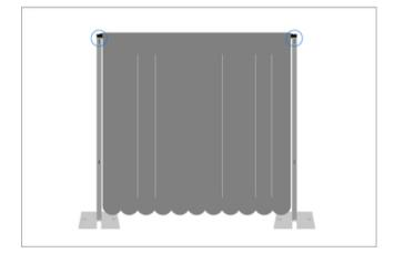
4 Attach each Hook End of the Drape Support to the top of the Upright
