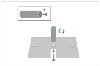
1) Remove the screw from the bottom of the pin. Place the screw through the desired pin hole on the base and tighten the pin until secure.
